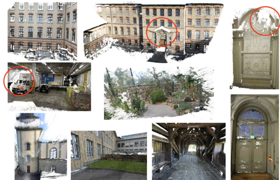
Figure 2.2: Example 3D reconstructions using PatchMatchNet [60] (MVS) on ETH3D benchmark [49], highlighting artifacts in the model.
